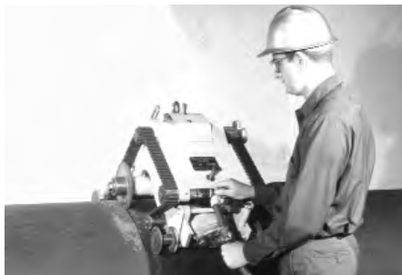
Cutting ductile iron pipe with milling cutter.
