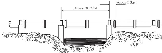
Case #2 uses 19'-3" lengths of flange plain end and flange bell (Fastite, MJ, or other push-on restrained) pipe. (MJ pipe is not available over 12" in diameter.) Since Case #2 uses flanged pipe joints, minimum nominal thicknesses shown in AWWA C115 are required.
