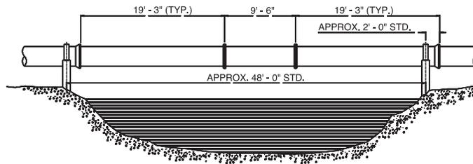
Case #3 uses 19'-3" lengths of flange bell and flange plain end pipe with a 9'-6" flange-flange pipe in the center. This can result in more mid-span deflection than Case #2 and, therefore, it is normally used only in 18" and larger sizes.
