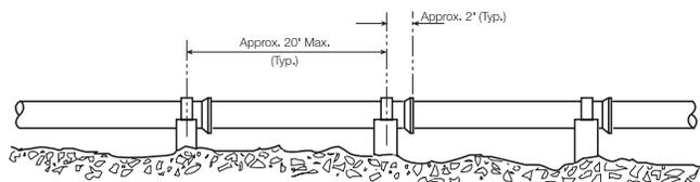
Case #1 uses 20' or less lengths of Fastite, MJ, or other push-on restrained pipe. (See page 7-29 General Note 3.) This length is normally subject to normal manufacturing and trim (cut pipe) variations, with some pipe allowed up to two feet shorter than full length. Where exact length pipe is required, say to fit existing pier spacings, etc., contact AMERICAN.
